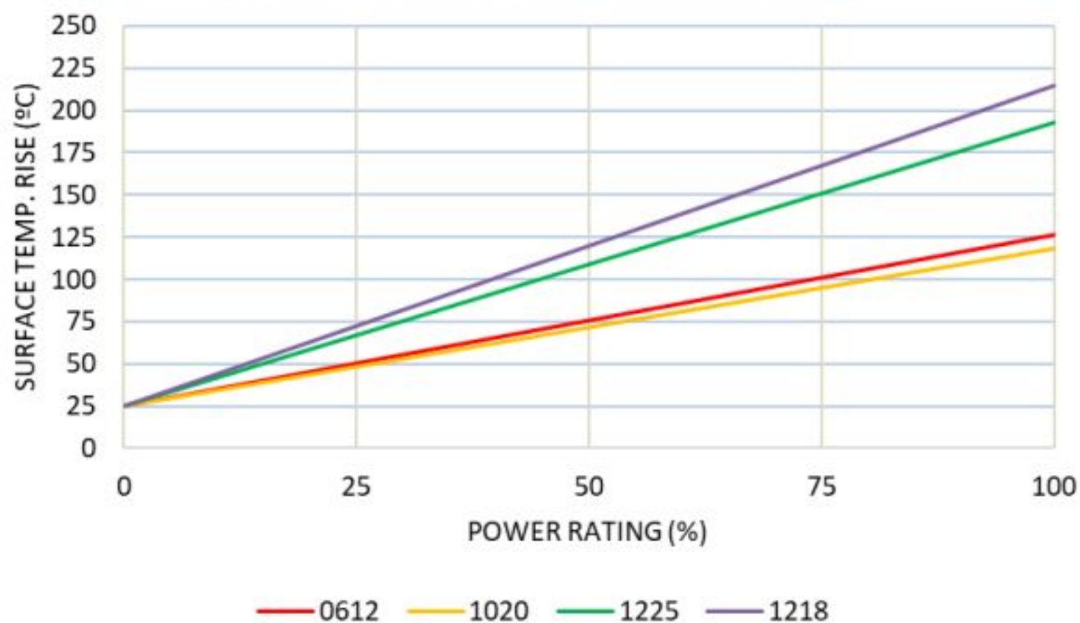
Surface Temperature vs. Power Rating
