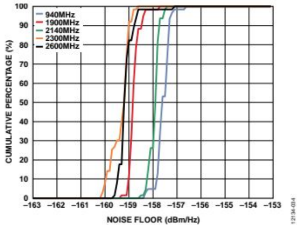
Figure 34. Noise Floor Cumulative Distribution at Various LO Frequencies Using Internal LO; I/Q Input with 500 mV DC Bias and No RF Output
